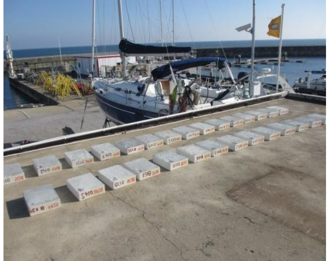
Concrete slabs exposed to chloride attack in severe real environments
